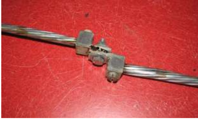
Figure 1: Typical connector sample. Aluminum wire and AL/CU dual-rated connector shown.
