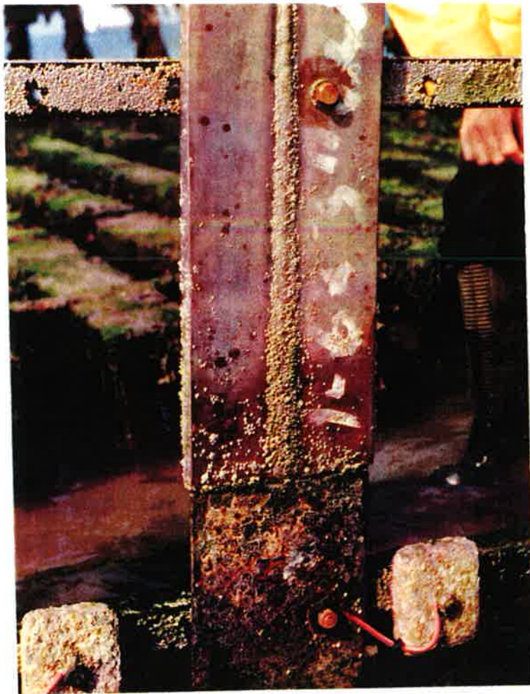
Figure 17. 90-10 copper nickel and 50D steel after 16 weeks on the half tide site.
