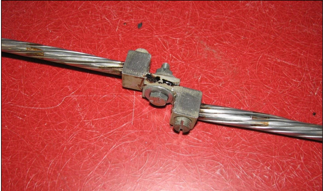
Figure 1. Typical connector sample (AL/CU dual rated shown).
