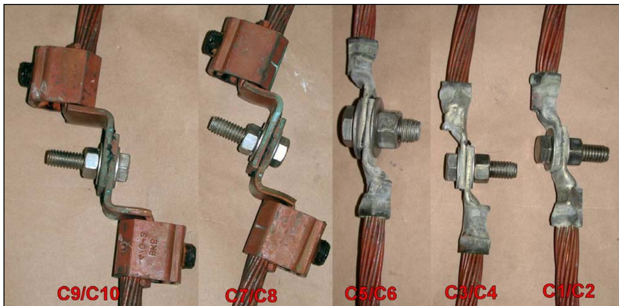
Figure 18. Copper samples after 1000 hours of testing.
