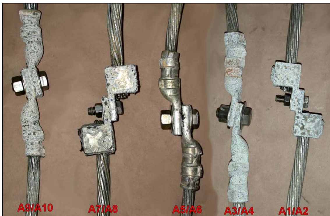
Figure 7. Aluminum-to-aluminum samples after 1000 hours of testing.
