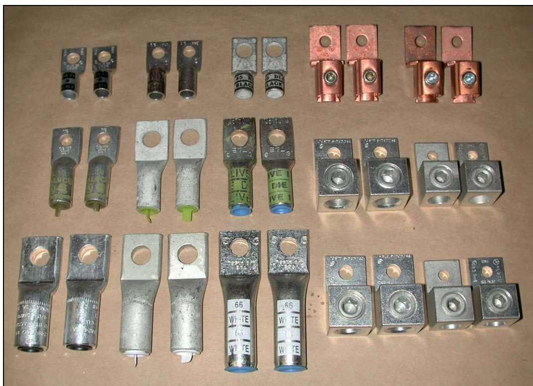
Figure 1. Connector samples used for corrosion and current burst testing.
