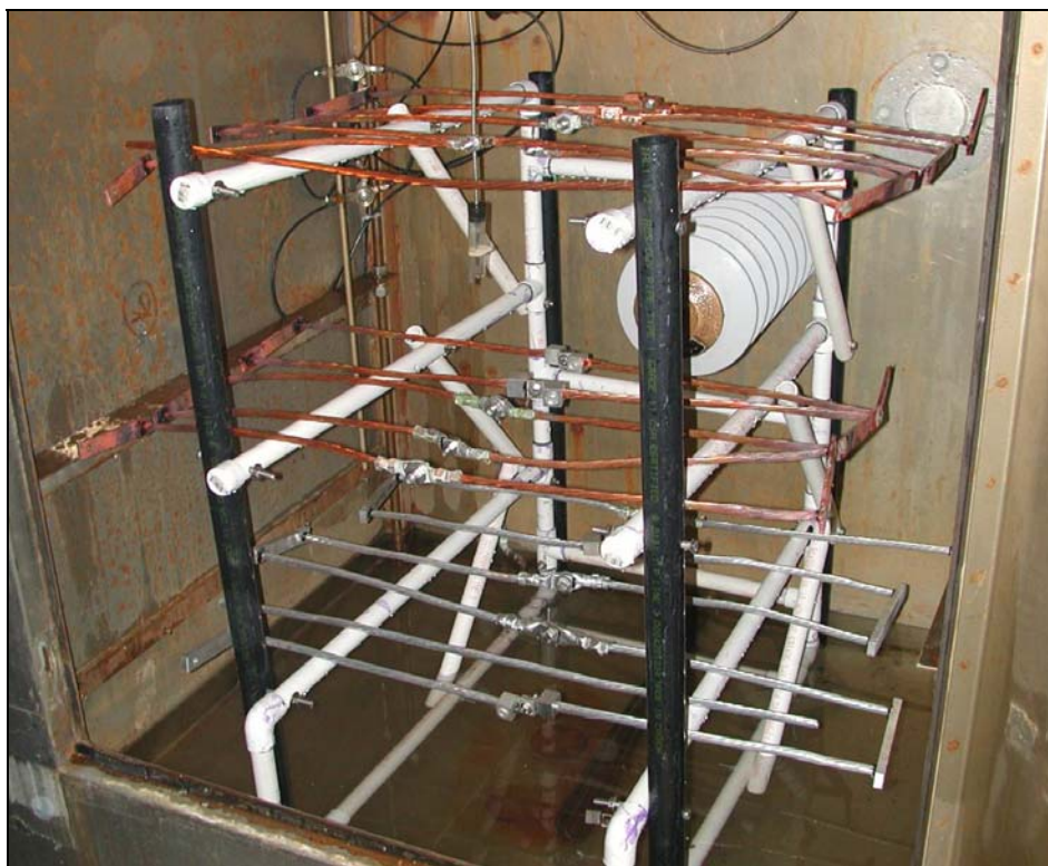
Figure 5. Connector samples set up in the weathering chamber.
