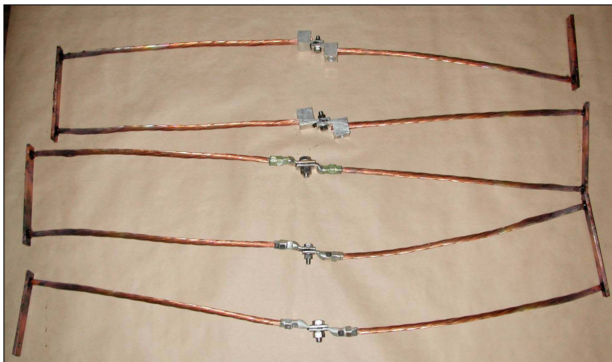
Figure 4. Connector sample assembly with equalizers and conductor (copper conductor/aluminum connector samples shown).
