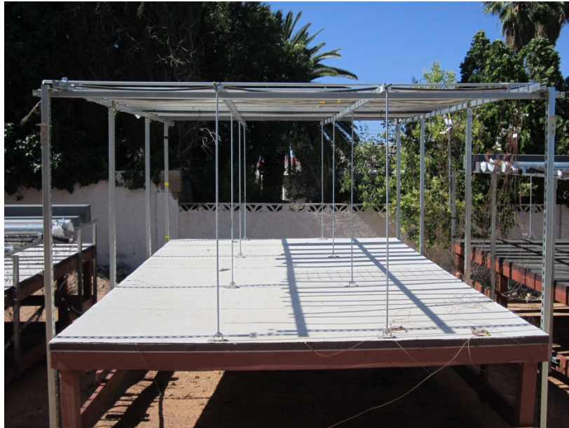
Fig. 2 – Wiring Systems Mounted 5 Feet off Roof
