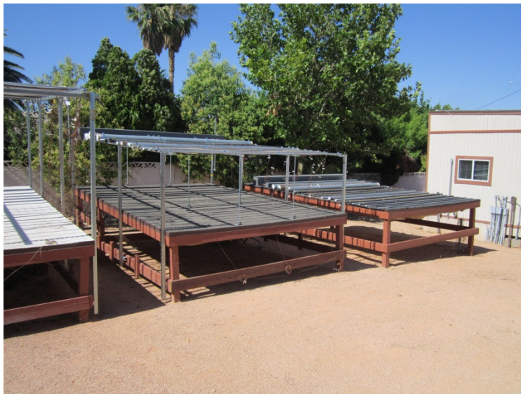
Fig. 1 – Wiring Systems Mounted 3 Feet off Roof
