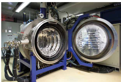
Figure 19 – Vacuum soldering/brazing furnace [30]
