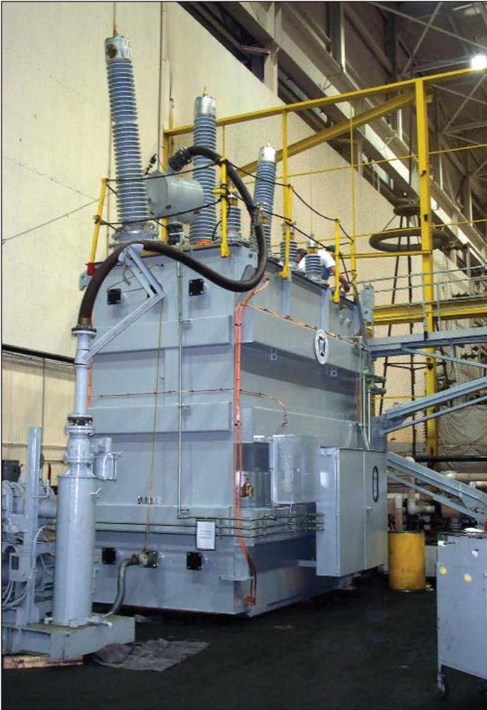
*Figure 2. A 400-MVA, 495,000-lb transformer under construction at PTTI. The company uses copper exclusively in all its transformer product lines.*
