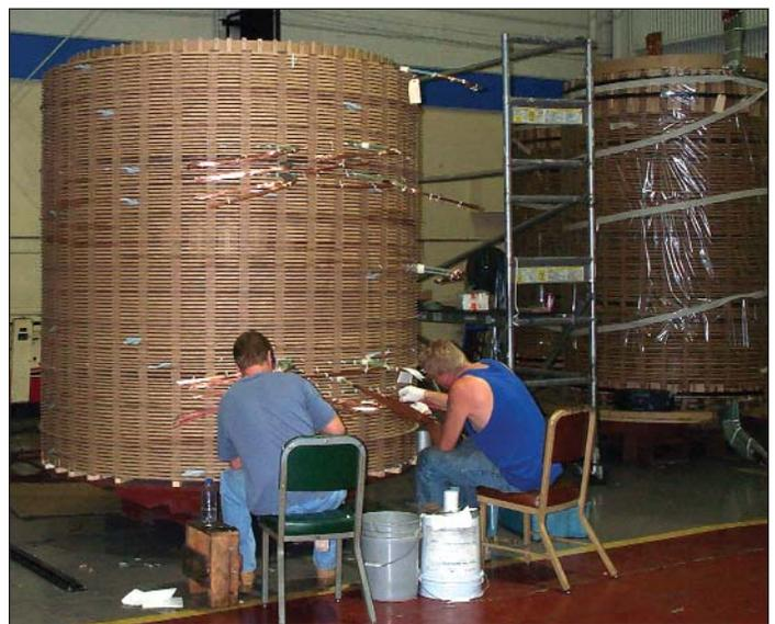
*Figure 4. Workers complete assembly of a large coil at Pennsylvania Transformer Technology Inc. With smaller conductors and good connectivity, copper is considered to have better manufacturability and, therefore, higher reliability than aluminum.*
