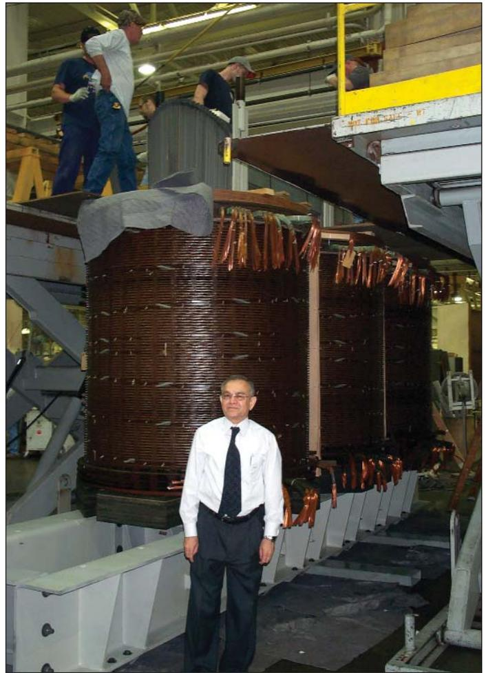
*Figure 1. Ravi Rahangdale, president of PTTI, stands before the 90,000-lb copper coils for a 150-MVA auto transformer. Copper's high volumetric conductivity helps keep the size of what will be a 405,000-lb unit manageable.*
