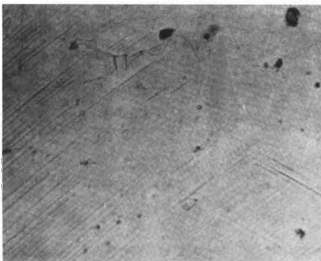
Figure 4. Microstructure of a single-phase (alpha) copper-tin alloy (88Cu-8Sn-4Zn). Structure shows slip lines. Note also traces of the delta phase (darker islands) (Reference 2).
