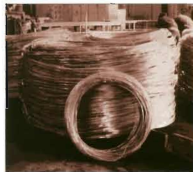
Figure 9 - A 10,000 lb. (4535 kg) copper coil produced by continuous casting dwarfs a coil produced from a single 250 lb. (113 kg) wire bar.
