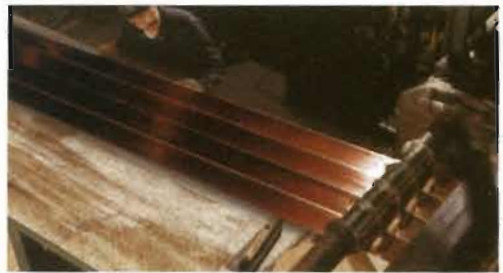
Figure 15 - Precision Slitting of Brass Sheet into Strip.
