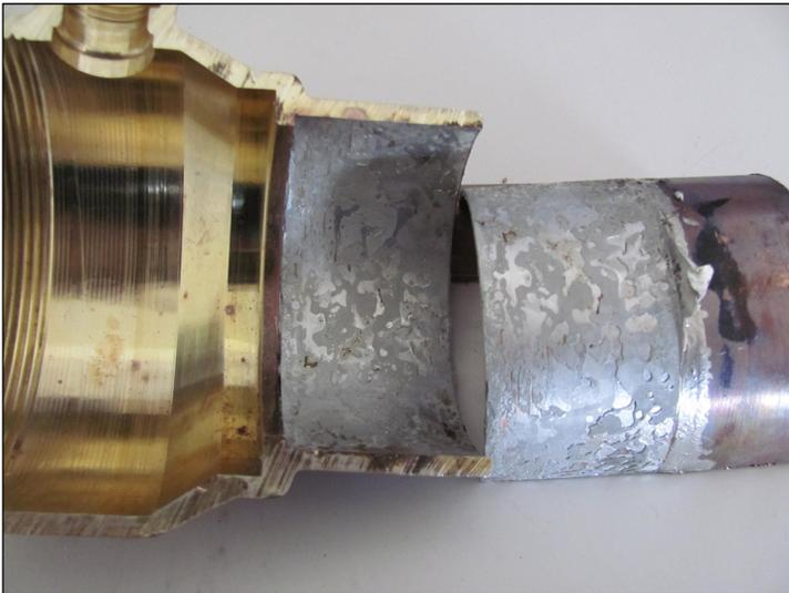
**Figure 3:** Properly Completed Solder Joint – Prepared identically to **Figure 1**. Brush marks from mechanical cleaning (stainless steel fitting brush inserted in power drill) no longer evident as proper heating allowed for complete solder flow and fill in the capillary space.
