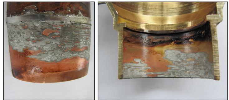
**Figure 2:** *Improperly Heated Solder Joint – Incomplete solder flow in the capillary space due to inadequate preheating of the tube surface.*
