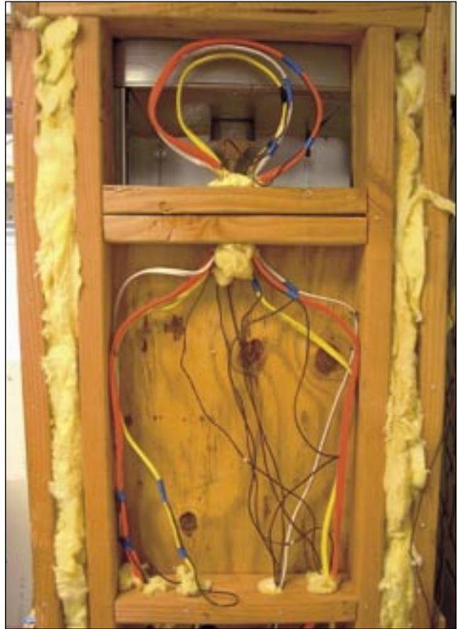
**Figure 13. Bundle experiment, including instrumentation wiring, in test rig**
