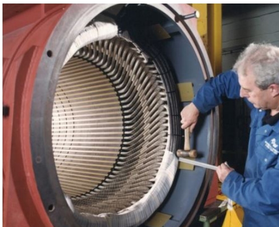
Above: Copper windings being installed in a stator/rotor for a low-speed direct drive (no gearbox) Enercon wind turbine generator (source: Enercon.de). Below: copper windings in more common high-speed gearbox-connected generator (Source: rjweng.com)
