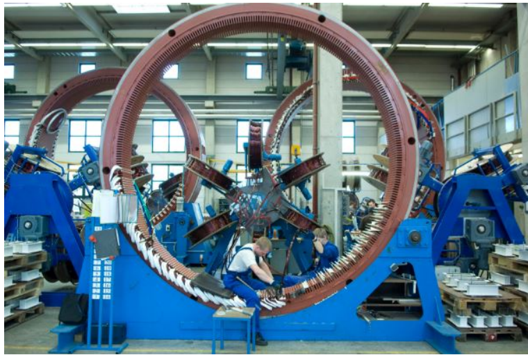
Above: Copper windings being installed in a stator/rotor for a low-speed direct drive (no gearbox) Enercon wind turbine generator (source: Enercon.de). Below: copper windings in more common high-speed gearbox-connected generator (Source: rjweng.com)
